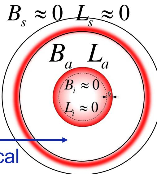
$$L_a' = \frac{L_a}{l} = \frac{\mu_0}{2\pi} \ln\left(\frac{r_2}{r_1}\right) = 241 \text{nH/m (RG58)}$$
