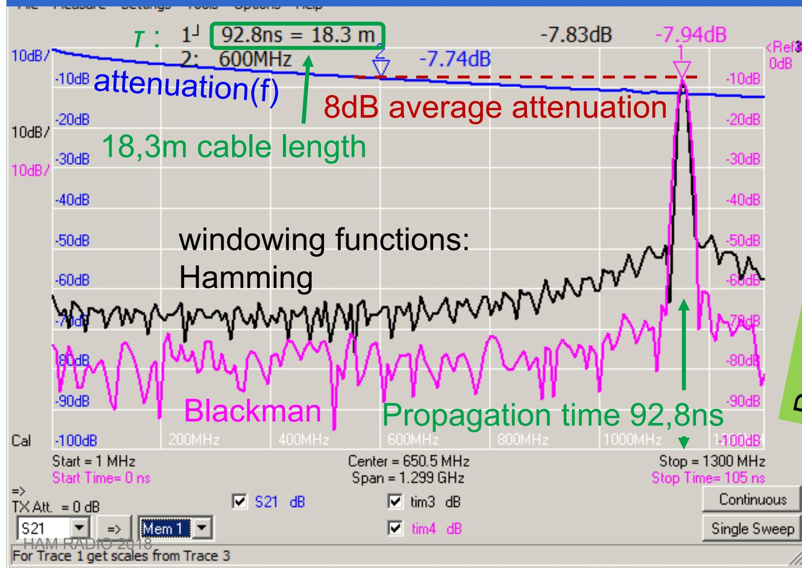
Determine either cable length or velocity factor
