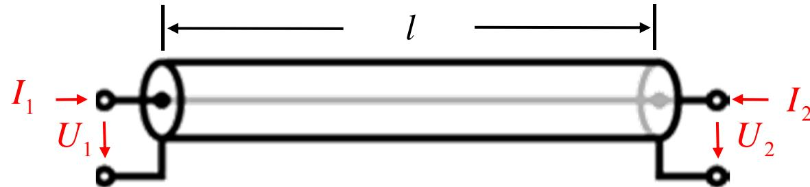
$$\begin{pmatrix} U_1 \\ U_2 \end{pmatrix} = \underbrace{\frac{Z_L}{\sinh(\gamma l)} \begin{pmatrix} \cosh(\gamma l) & 1 \\ 1 & \cosh(\gamma l) \end{pmatrix}}_{\text{Z-matrix}} \cdot \begin{pmatrix} I_1 \\ I_2 \end{pmatrix}$$
